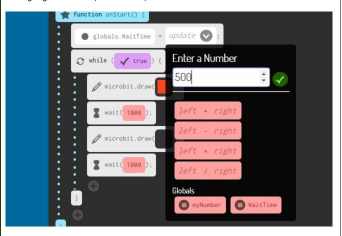
Now our variable **WaitTime** is set to **500** but we are not using it. So in the **wait** chunk after we've turned the LEDs on, click on the **number** (1000 in the picture above) and look at the bottom of the menu that appears, our variable **WaitTime** is available to select. Click on it to change the fixed number to our variable.
