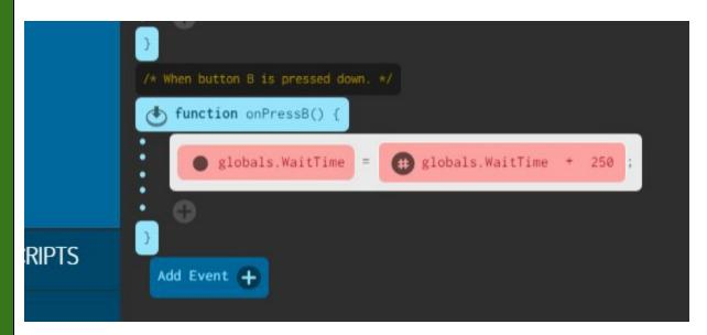
Now run your code. The LEDs will start flashing every half a second (500 milliseconds). Press **button B** (you can click on it on the simulator) and the speed they flash will slow down.
