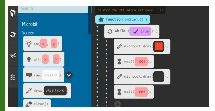
Run the code in the simulator and on the Micro:bit if you can.
