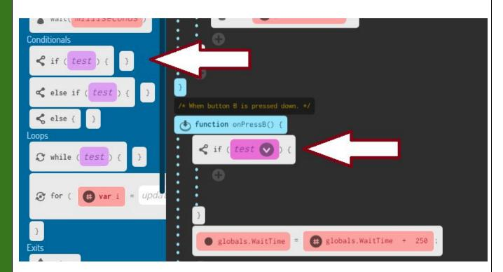
We only want to add to **WaitTime** if it's smaller than 5000 milliseconds, so on the **drop down menu** select the **left < right**:
