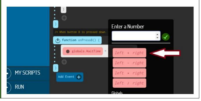
We now have two **drop down menus**. Lets add 250 milliseconds to **WaitTime** everytime the button is pressed. So we want to end up with **WaitTime=WaitTime + 250**.
