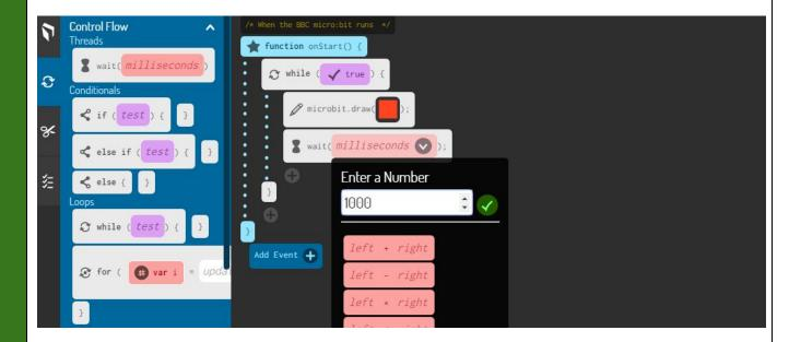
When a chunk needs more information like the wait chunk, the information is called a parameter. The wait chunk's parameter tells it how long to wait for until letting the code continue. Because we can have really short times to wait, its parameter is in milliseconds. There are 1000 milliseconds in a second so the code above will wait for 1 second.
